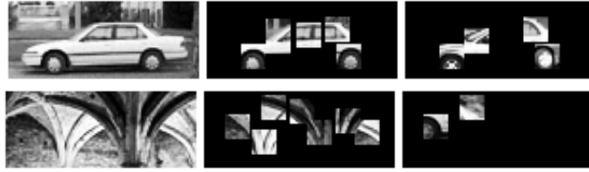
Fig. 4. Examples of the part detection process applied to a positive and a negative image during training. Center images show the patches highlighted by the interest operator; notice how this successfully captures the interesting regions in the image. These highlighted interest patches are then matched with vocabulary parts. In the right images, the highlighted patches are replaced by an arbitrary member of the part cluster (if any) matched by this detection process. These parts, together with the spatial relations among them, form our representation of the image.
